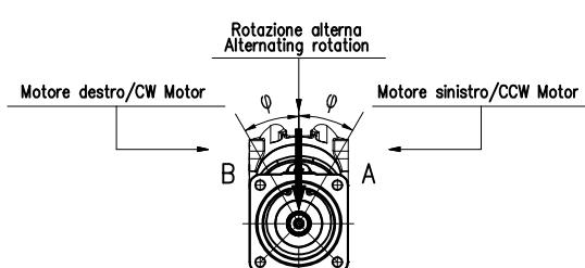
The bearing operating life increases up to 30% when the load is applied with some peculiar directions and the maximum increase is dependent on the operating pressure and the nominal size of the unit.
