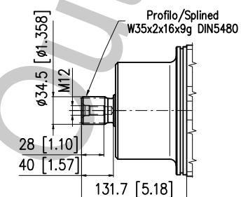
S1, S2: Drenaggi / Drain ports - 1/2 G (BSPP)
