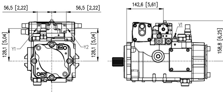
Y1-Y2: Attacchi pilotaggio comando / Control piloting pressure ports - 1/4 G (BSPP) (ISO)
