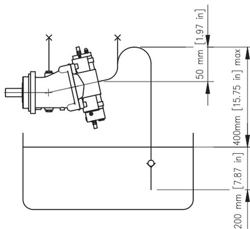
Figura 3 - Installazione H1V / Figure 3 - H1V installation
