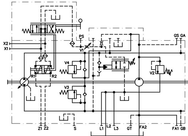
Note: The pressure compensator valve can be combined with electric cut-off (EP) valve.
