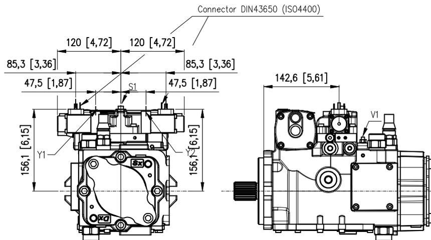
Y1-Y2: Attacchi pilotaggio comando / Control piloting pressure ports - 1/8 G (BSPP) (ISO)
