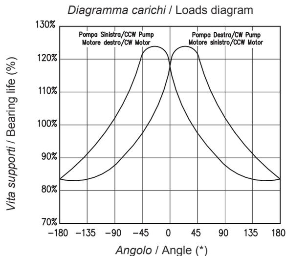
Figura 7.1 - Carichi radiali / Figure 7.1 - Radial loads
