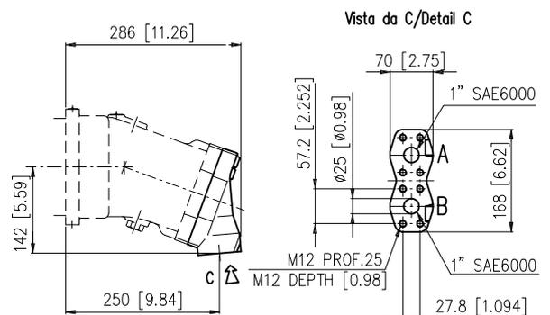
**S1, S2: Drenaggi (1 tappato) / Drain ports (1 plugged) - 1/2 G (BSPP)**
