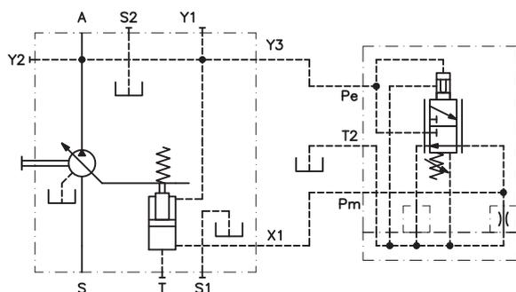
The constant pressure control of the pump can be remotely piloted by means of the internal pilotage sequence valve VSI (see valves and accessories section). VSI valve is directly assembled on pump, but it also can be ordered separately. Setting adjustment is 50 bar [725 psi] to 350 bar [5075 psi]; the piping length should not exceed 5 mt [16ft]. Port T2 (fixed restrictor) must be directly connected to the tank and circuit relief valve must be 30 bar [435 psi] higher than the PCR control.
