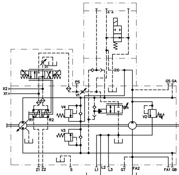
Note: The electric cut-off valve can be assembled on standard S6CV pump and it can be combined with PC (EP) valve
