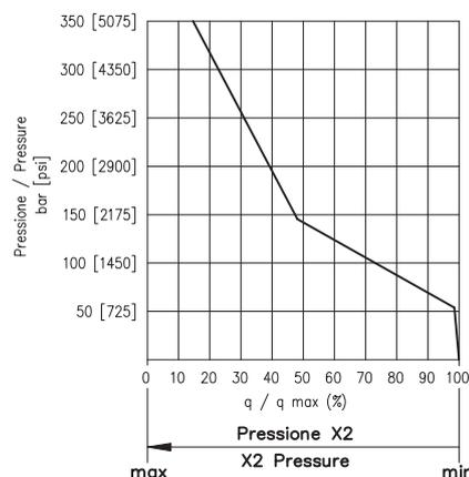
**Control boosting:** When it is necessary to change the displacement of the pump with a working pressure lower than 40 bar [580 psi], the control must be boosted by means of an auxiliary circuit connected at Y3 port.
