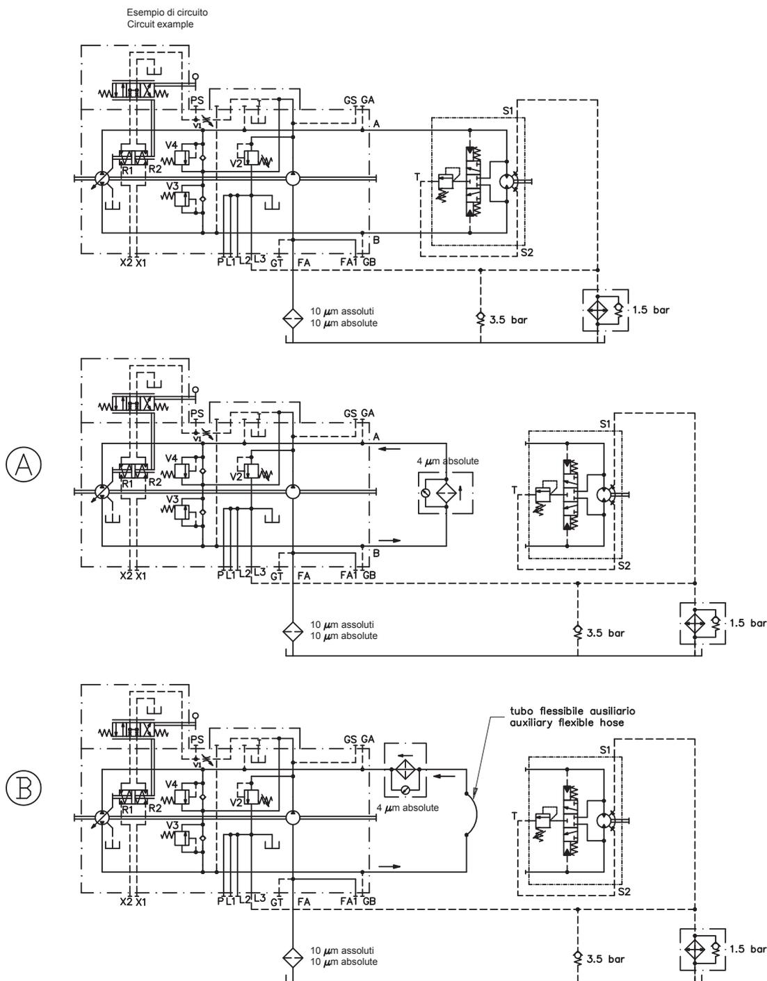
Figura 5 - Lavaggio circuito chiuso / Figure 5 - Closed circuit cleaning
