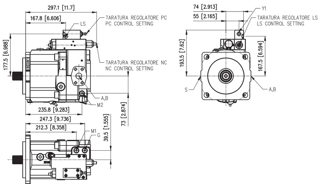
LS: Attacco pressione Load Sensing / Load Sensing Pressure port - 1/8 G (BSPP) Prof./Deep 10 [0.393]
