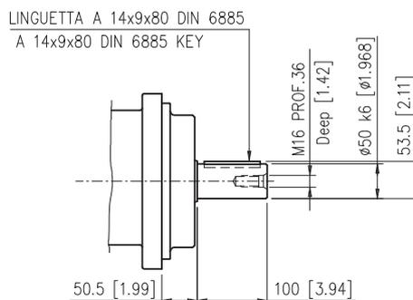
S1, S2: Lavaggio (tappati) / Flushing ports (plugged) - 1" 1/16-12 UN 2B
