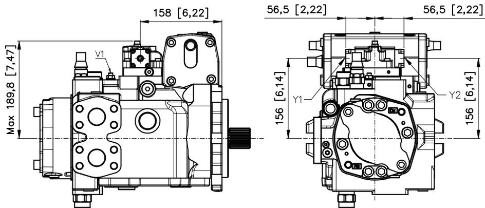
Y1-Y2: Attacchi pilotaggio comando / Control piloting pressure ports - 1/4 G (BSPP) (ISO)
