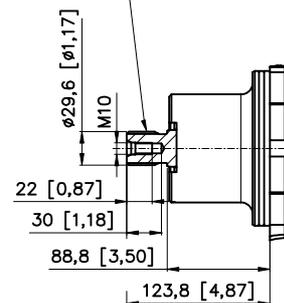
S1, S2: Drenaggi / Drain ports - 1/2 G (BSPP)
