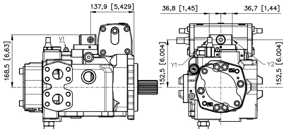
Y1-Y2: Attacchi pilotaggio comando / Control piloting pressure ports - 1/4 G (BSPP) (ISO)
