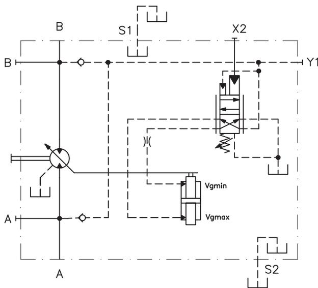
The hydraulic limiting device makes possible to reduce the pressure setting of RPE control by means of an external pilot pressure applied at port X2. The RPE control pressure setting is reduced proportionally to the pilot pressure in the ratio of 1/17 (for each pilot pressure bar, the preset operating pressure is reduced of 17 bar) [170 psi each 10 psi of pilot pressure]. Max permissible pilot pressure at port X2 = 100 bar [1450 psi].
