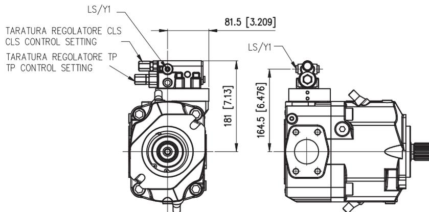
LS: Attacco pressione Load Sensing / Load Sensing Pressure port - 1/8 G (BSPP) Prof./Deep 10 [0.393]
