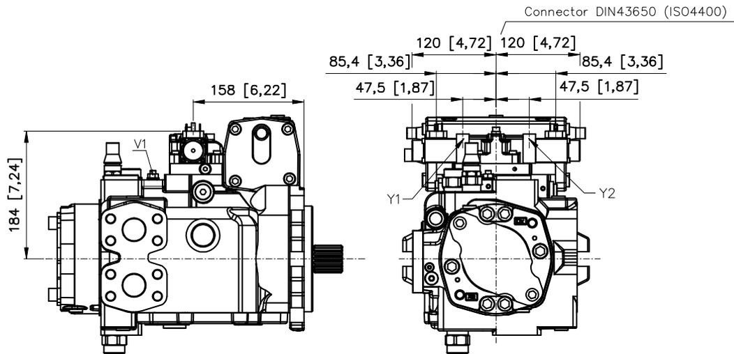
Y1-Y2: Attacchi pilotaggio comando / Control piloting pressure ports - 1/8 G (BSPP) (ISO)
