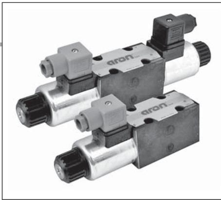
The open loop valves of series XDP... control the direction and the volume of the flow according to the feeding current to the proportional solenoid. By using a valve body equipped with increased passage channels it is possible to reach the highest capacity of its dimensions at a parity of pressure drops, (40 l/min with  $\Delta p$  of 10 bar).
