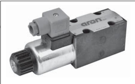
The open loop proportional flow regulator is 2 and 3 way compensated with priority function. It is designed to regulate flow in proportion to an applied electrical current (REM or SE3AN power amplifier). Flow regulation is load independent - B port. Load compensation is achieved by a spool compensator which holds the pressure drop constant across the proportional spool.
