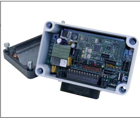
The Self leveling Device LAB3 meets the safety requirements:
